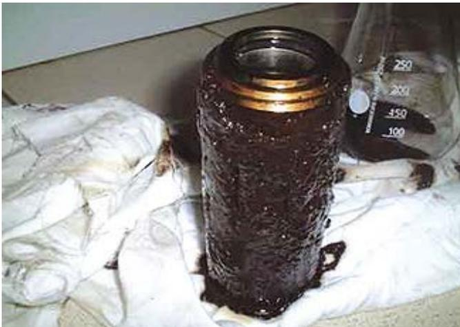
**Consequences of Varnish and Oil Degradation**
