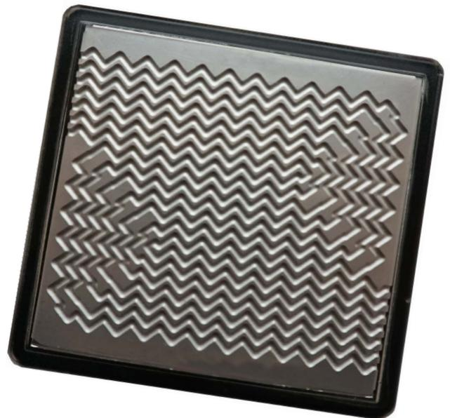
▶ This plate illustrates the inside of a heatric cooler. A huge amount of plates similar to this one are compressed. During production, gas and coolerwater navigate through the tiny corridors independently from eachother until clogged.
