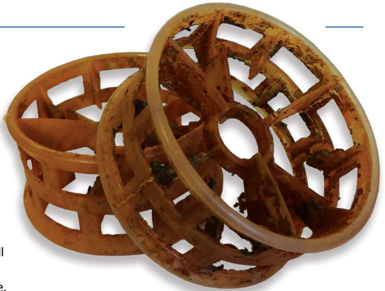
▲ *"Tower Packing Rings" before undergoing their chemical cleaning. It is clear to see how dirty the rings are, as well as the number of nooks and crannies, where oxygen bubbles and other issues may form, meaning filtering is reduced.*
