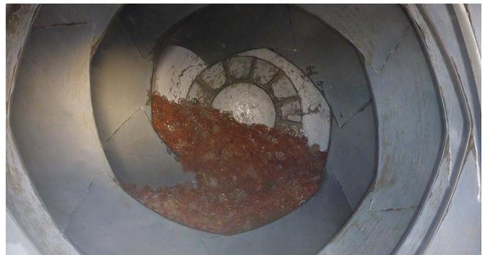
▲ "Tower Packing Rings" being chemically cleaned inside the cement mixer.
