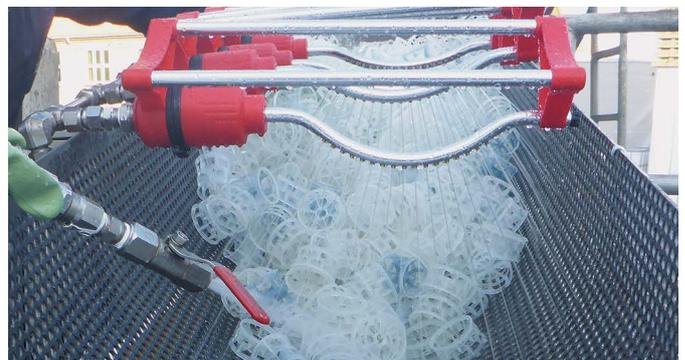
▲ The chemically cleaned "Tower Packing Rings" are rinsed from chemicals by three garden sprinklers.
