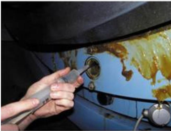
**Picture 2** – Picture of an over-greased bearing, where the fresh grease has been forced out of the bearing seals.
