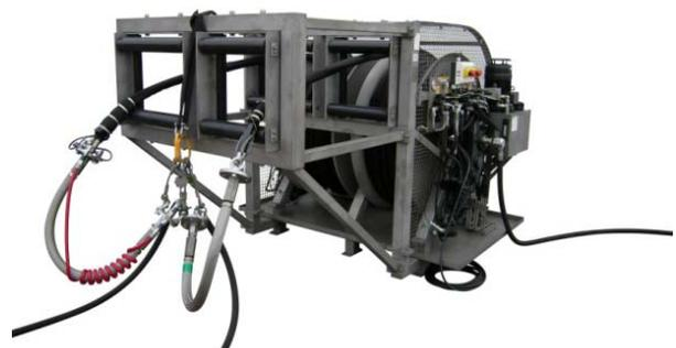
A wave-compensating Hose Reel is connecting the equipment at the service vessel with the platform.
