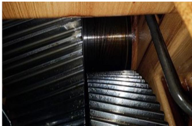
▲ Before up-tower flushing; interior covered in varnish
