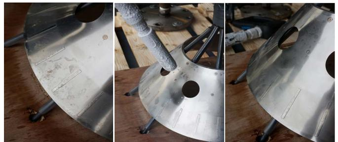
▲ *Stuck and burned oil and dirt prevent ceramic coating. These visuals show one of the centrifugal dishes prior to, during and after iceblasting.*
