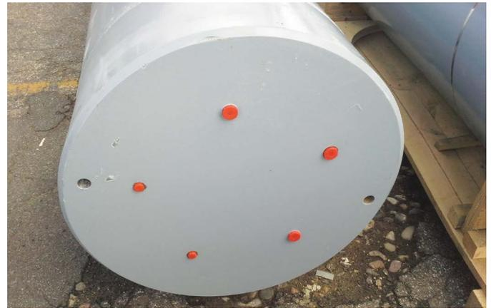
▲ *Incorrect sealing of the bottles by using the wrong vents and seals enabled saltwater and moisture to penetrate and thereby cause the rust.*
