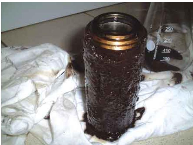
Picture 2 - Plugged Filter from a large-frame industrial gas turbine.
